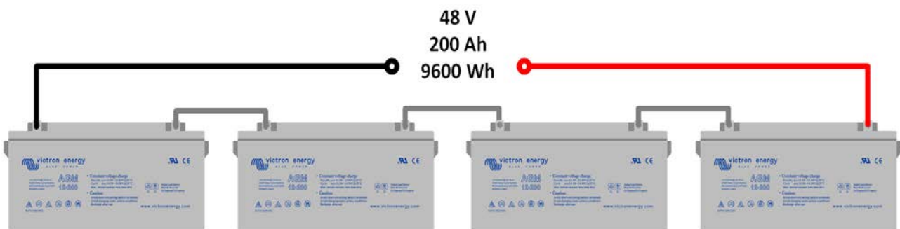
Four batteries in series
