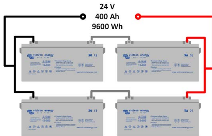
Four batteries in series/parallel
