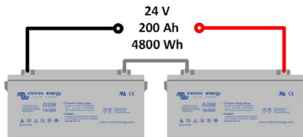
Two batteries in series
